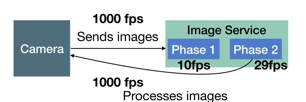
• When adding multiple pipelined components -> throughput is the minimum value
